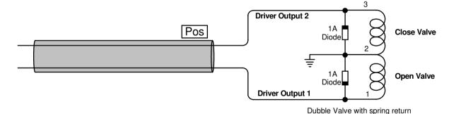
**NB!!** The Diode must be connected. Make sure the stripe on the diode is facing the positive.
